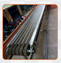
Chain conveyors are used to convey heavy unit loads, like pallets, grid boxes and industrial containers. Chain conveyors are with single or double chain strand in arrangement. The load is placed on the moving chains. The chain conveyors are used in forging industry, Furness, surface treatment, heat treatment plants etc.
